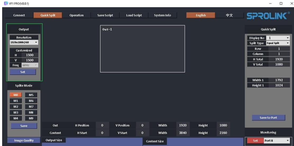
2. Setup the Quick Split parameters. VF1 PRO support equal and unequal split. Set the proper parameters the device will calculate the output port parameters automatically and display the proper image.
