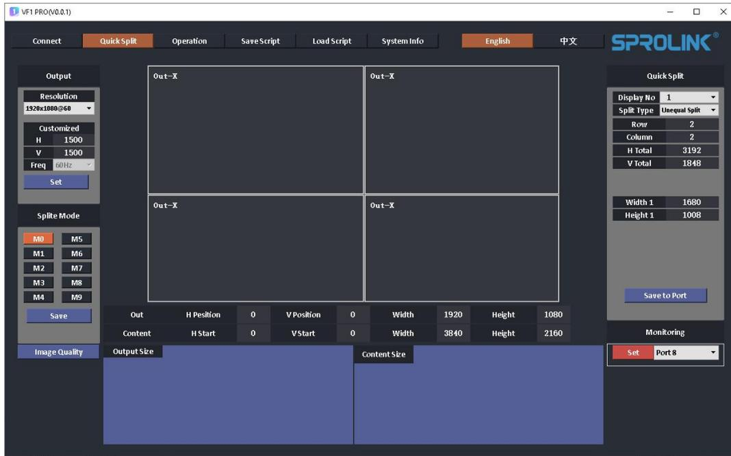
3. Choose Out-X one by one and arrange proper output port according to the cabling.
